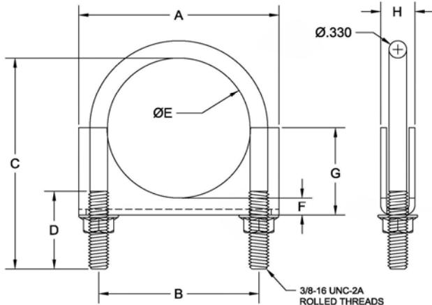
UDO Series Clamps Includes: 3/8-16 Round U-Bolt, Double Edge, Open End Saddle and (2) Serrated Flange Nuts
