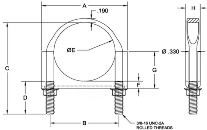
UFDO Series Clamps Includes: 3/8-16 Flat U-Bolt, Double Edge, Open End Saddle and (2) Serrated Flange Nuts
