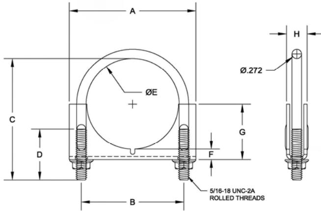
PC Series Clamps Includes: 5/16-18 Round U-Bolt, Double Edge, Open End Saddle and (2) Hex Nuts
