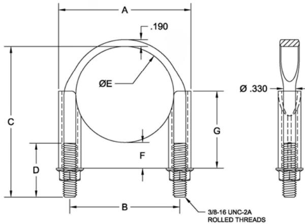
UF Series Clamps Includes: 3/8-16 Round U-Bolt, Single Edge, Guillotine Saddle and (2) Serrated Flange Nuts
