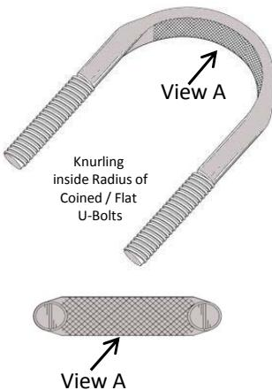
Some of the Flat / Coined U-Bolts have knurling on the inside bend radius of coined / flat U-bolts. This is now available on most sizes of coined / flat U-bolt clamps. This knurling feature will provide:
