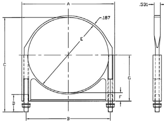
AUF Series Clamps Includes: 3/8-16 Flat U-Bolt, Heavy Duty Cast Aluminum Saddle and (2) Serrated Flange Nuts
