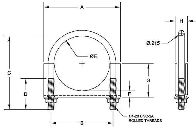
AC Series Clamps Includes: 1/4-20 Round U-Bolt, Double Edge, Open End Saddle and (2) Hex Nuts
