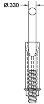
U Series Clamps Includes: 3/8-16 Round U-Bolt, Single Edge, Guillotine Saddle and (2) Serrated Flange Nuts
