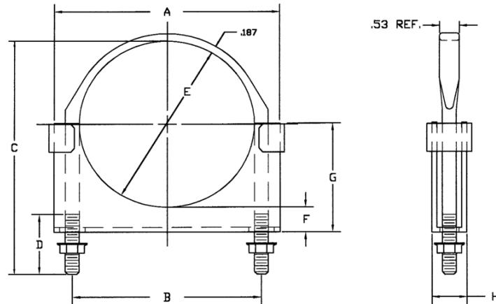
UFD Series Clamps Includes: 3/8-16 Flat U-Bolt, Double Edge, Closed End Saddle and (2) Serrated Flange Nuts
