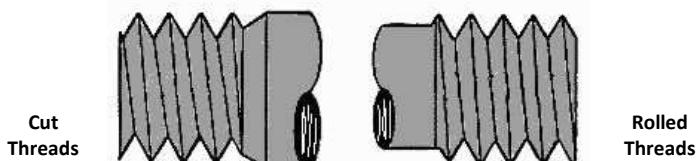
The average material savings for a thread size of 3/8-16 is 26 to 28 percent. The rolled thread process uses dies that are extremely accurate allowing a pitch diameter tolerance of .001 inches. Rolled threads are faster to produce, with less labor cost than cut threads and are more resistant to damage during handling.
