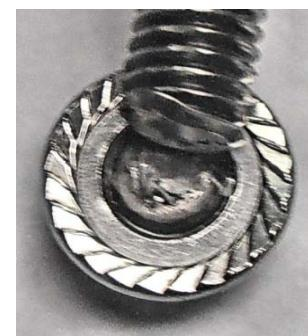
Galling can be minor causing only slight damage to the threaded surface. In severe cases, it can completely weld the nut and bolt together and prevent the removal of the fastener. Often times, during installation the threads may strip out or the fastener may twist off. Galling is more likely to occur when the external threads are cut, rather than rolled. Cut threads have rougher surfaces due to the machining process. Galling can also result from surface oxidation in some materials.
